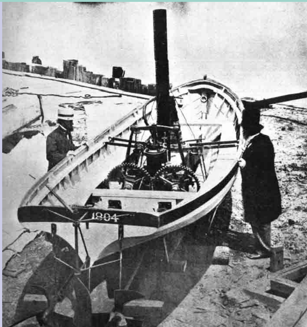
1860s replica of John Steven's 1804 steam-powered motorboat, with twin counter-rotating propellers.
